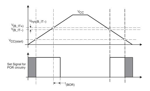
As the  $V_{(B\_IT\_)}$  level is significantly above the  $V_{min}$  level of the POR circuit, the BOR provides a reset for power failures where  $V_{CC}$  does not fall below  $V_{min}$ . See device-specific datasheet for parameters.
